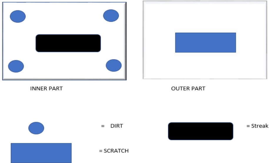
Figure: Defect Concentration Diagram for car window shield
