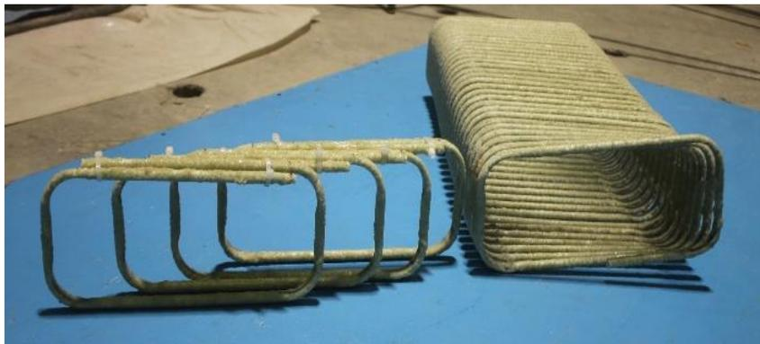
**Fig. 4: GFRP stirrups as shear reinforcement [3]**
