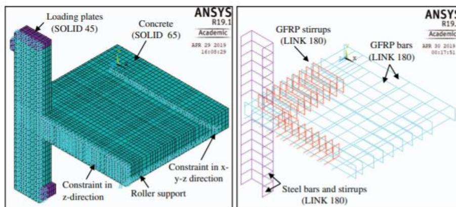
Fig. 9. Geometry and reinforcement details of ANSYS model [24].
