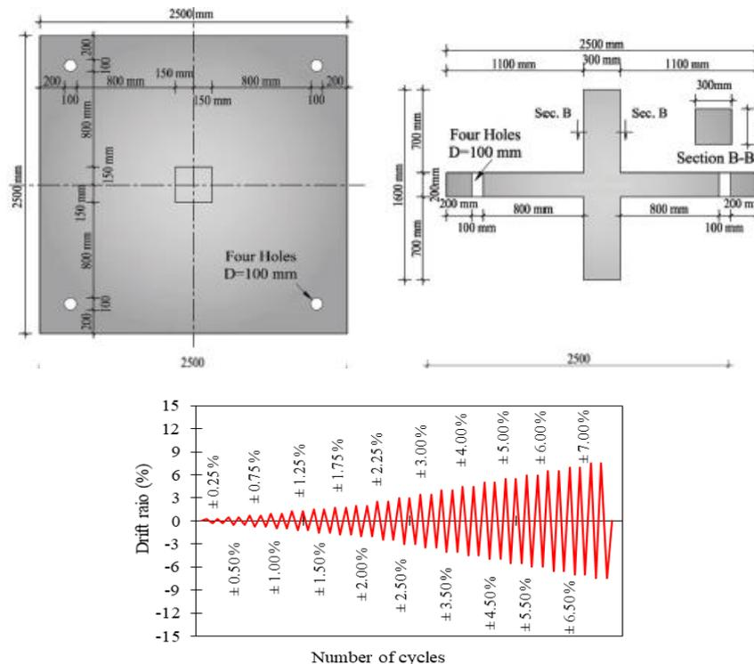
**Fig. 5: test specimens' geometry and loading routine [16],[17],[18]**
