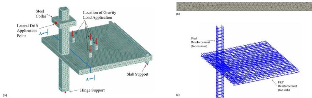
**Fig. 10. Typical details of FEM: (a) macroelements and boundary conditions; (b) mesh discretization at Section A-A; and (c) discrete reinforcement [25].**
