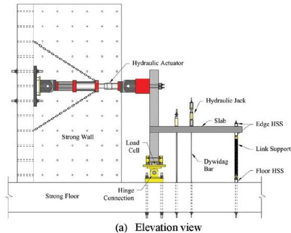
**Fig. 6 : Schematic test setup [21].**
