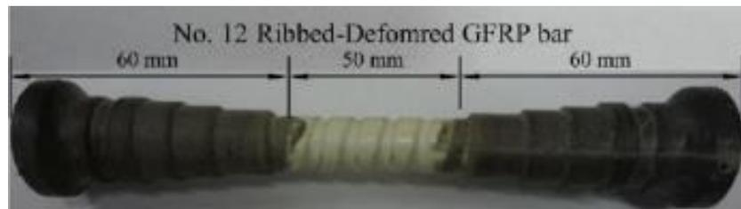
**Fig. Error! No text of specified style in document. : Newly developed GFRP shear studs [8]**
