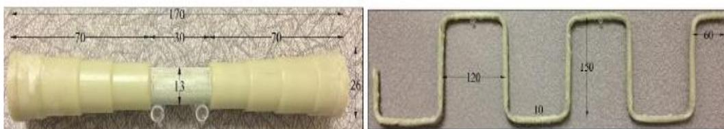
**Fig. 3: GFRP headed studs and GFRP corrugated bars [10].**
