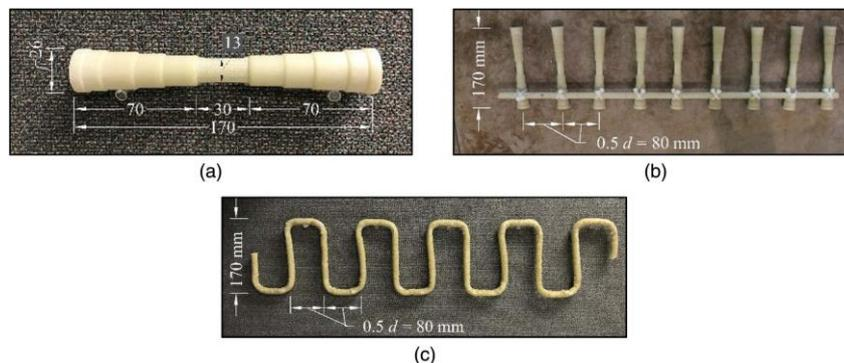
**Fig. 7 : GFRP shear reinforcement (dimensions in millimeters): (a) shear stud; (b) shear studs' rail; and (c) corrugated bar [21].**
