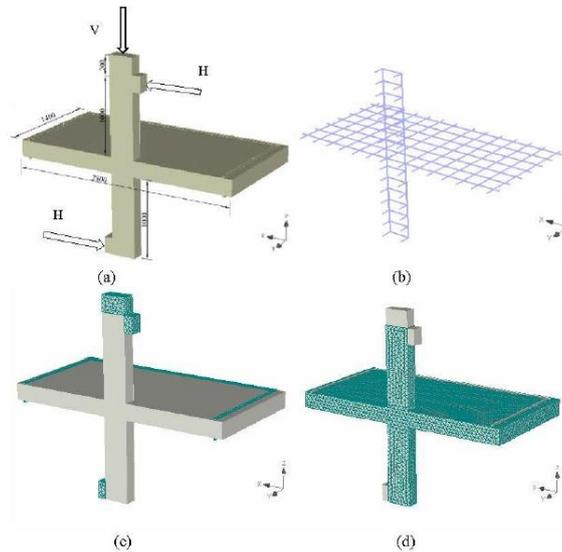
Fig. 8: ATENA-3D model. (a) Model geometry; (b) Reinforcement configuration; (c) Loading and supporting plates (meshed); (d) Slab and column (meshed) [9].
