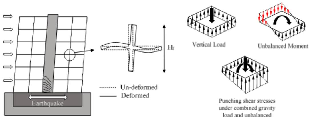
**Fig. Error! No text of specified style in document.: Punching stress under a combination of gravity and unbalanced moments**
