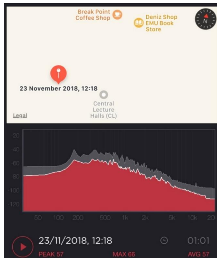
Fig 18: Graphically representation of background Noise estimated within an empty classroom (Door open)
